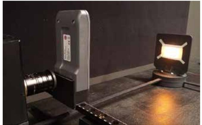
*MSC15 set up in front of the luminance camera to check the transmission spectrum.*
