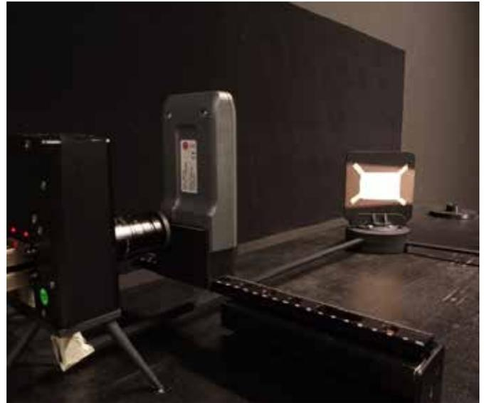
*Material illuminated from the side to check the reflection spectrum.*
