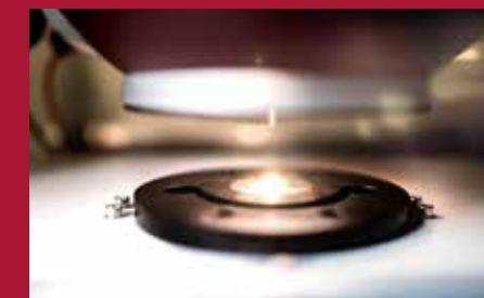
The TP121-TH LED testing system provides fully automated testing routines for SMD and on-board LED devices.
