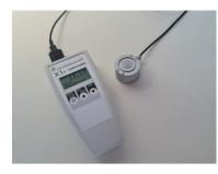
Mobile UV radiometer with separate measuring device and detector for measuring the irradiance and dose of germicidal mercury lamps.
