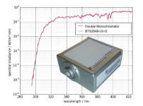
Comparison of UV solar irradiance measurement with BTS2048-UV-S and a double monochromator. Demonstrates similar scattered light rejection but with much reduced measurement time.
