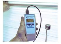
The X1-4 UV erythema meter is used in conjunction with the XD-45-ERYC detector to enable the on-site testing of sun tanning equipment.
