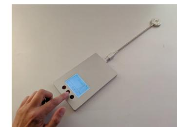
*BTS256-UV-4 hand-held measuring device with flexible detector head.*
