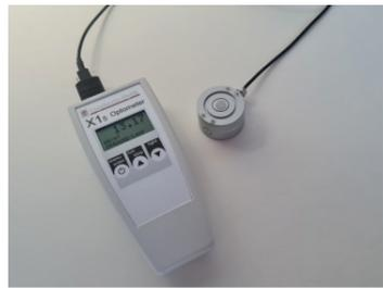
Mobile UV radiometer with separate measuring device and detector for measuring the irradiance and dose of germicidal mercury lamps.
