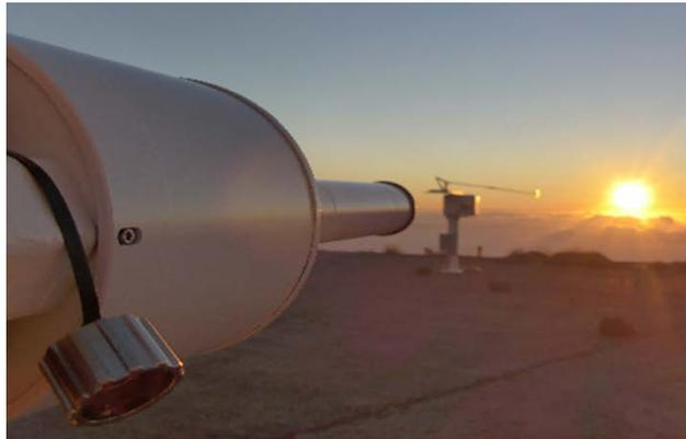
*BTS2048-UV-S mounted on a solar tracker*
