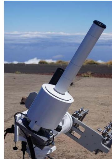
Ground-based spectroradiometer measurements of direct solar UV irradiance can be used to determine the Total Ozone Column (TOC) by applying the Beer-Lambert law in conjunction with the known absorption characteristics of ozone over the 290-350nm wavelength range. Suitable modelling is required to minimise the influences of other atmospheric attenuators [1].
