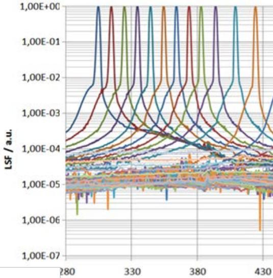
Line Spread Functions (LSF) form a signal distribution function (SDF) characterization matrix of the spectrometer.
