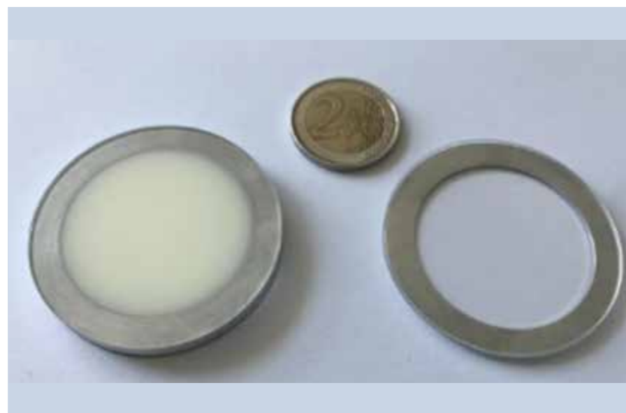
This picture shows some of the cuvettes for liquid samples. Solid samples should have similar geometry.
