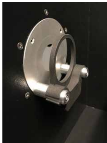
This picture shows the sample chamber where either solid or fluid samples (in cuvettes) could be mounted/clamped quickly and easily
