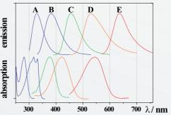
**KIT Spectral Emission Standards** little anisotropy, known stability & purity supply of dyes & solvent, cert. corr. emission spectra & SOP for use
