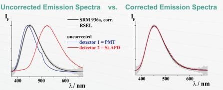
Emission spectrum of quinine sulfate dihydrate SRM936a measured with two detection systems before and after spectral correction and its corrected emission spectrum including uncertainty (RSEL)<sup>[1]]</sup> as certified by NIST<sup>[2]</sup>.
