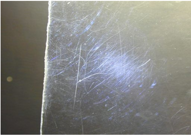
Plexiglas Window with Scratches
