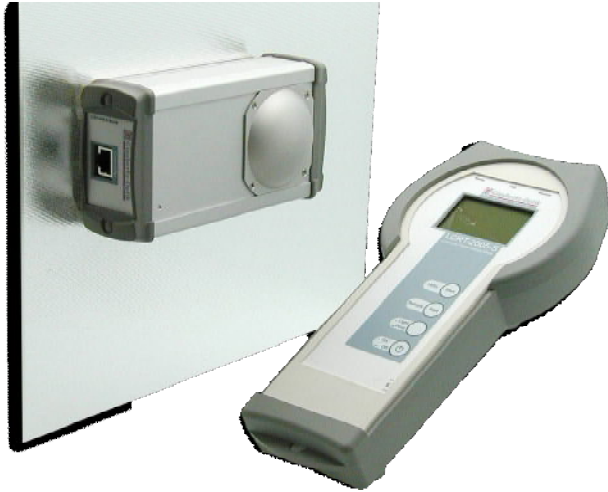
LCRT-2005-S Measuring Flat Glass Sample
