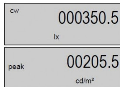
Large Digital Display with Measurement Unit and indication of cw or peak hold measurement mode
