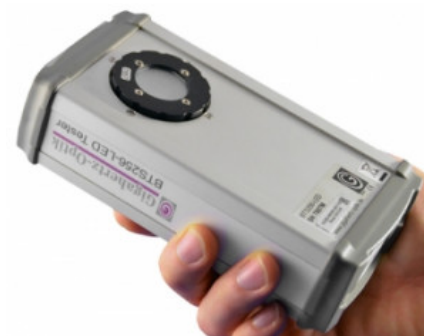
BTS256-LED with the BTS256-LED-DA diffusor window for illuminance measurements.
