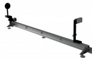
BTS256-LED spectroradiometer with the GB-GD-360-RB40-2 goniometer
