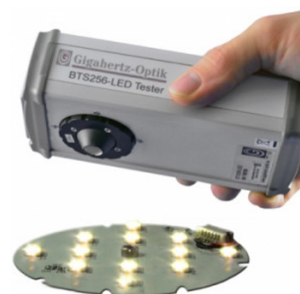
BTS256-LED for measurement of the luminous flux, spectrum, color, and color rendering index of single LEDs
