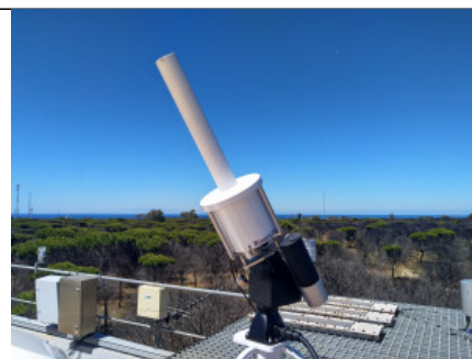
SUT-1711 equipped with BTS2048-UV-S-WP and tube for direct sun measurement
