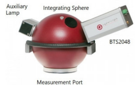
The BTS2048-UV can directly plugged on a integrating sphere (picture shows the constructional identical BTS2048-VL)
