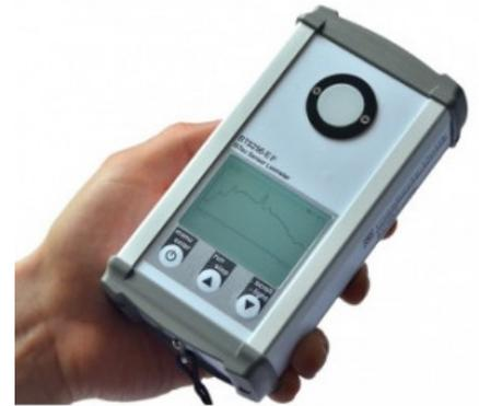
BTS256-EF for complex measurements in lighting technology, including flicker measurement
