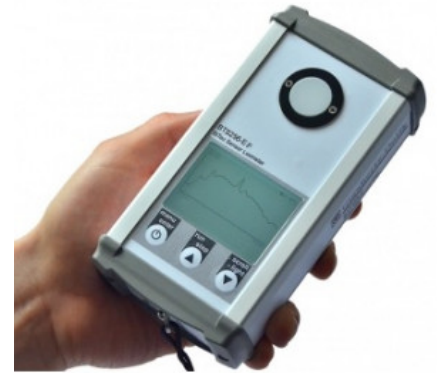
Spectral light meter with flicker measurement function
