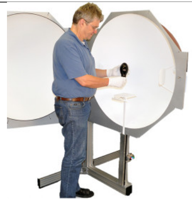
BTS256-LED Tester with 1m diameter integrating sphere
