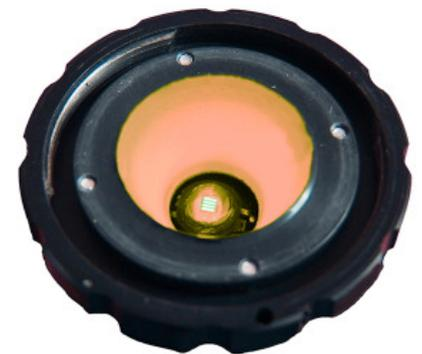
The conical measurement port is placed over the test LED and detects all the radiation in a 2pi space
