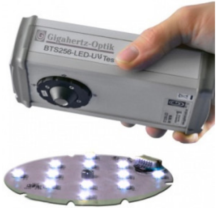
Compact UV LED spectroradiometer with internal integrating sphere
