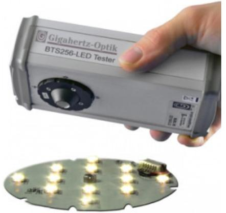
Compact spectroradiometer with internal integrating sphere
