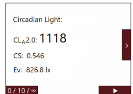
MSC15-CS for measurement of circadian stimulus, illuminance, spectrum and color
