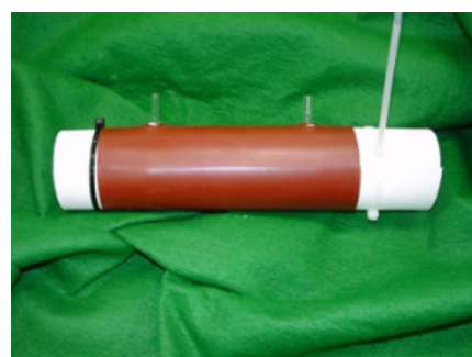
Picture 3: Custom design Integrating Sphere Source Insert
