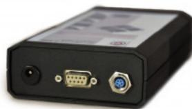
*The optometers P-9710 provide connections for power supply, detector heads with calibration data plug and a RS232 interface (from left to right).*
