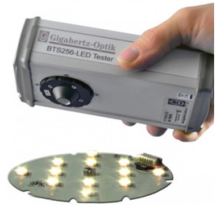
Compact spectroradiometer with internal integrating sphere
