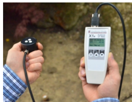
X14 being used for the measurement of UV radiation due to solar radiation.
